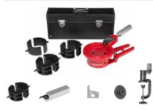
Robust pipe cutting machine made of metal for right-angled cutting of welded rain pipes of copper, titanium zinc, stainless steel, Ø 60–110 mm, welded drain/down pipes of stainless steel, Ø 50–110 mm.
