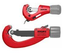
Compact, robust quality pipe cutter with cutting wheel and counter pressure rollers on needle bearings for thin-walled, stainless steel pipes, copper pipes and others, Ø 3-64 mm, wall thickness  $s \le 4 \text{ mm}$ .
