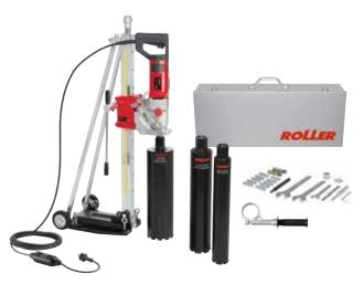
Universal, powerful, robust, handy diamond core drilling machine for core drilling for example in concrete, steel-reinforced concrete up to Ø 152 (200) mm, in masonry of all kinds, natural stone, asphalt, screed of all kinds, up to Ø 250 mm. For dry or wet drilling, hand held or with drill stand.
